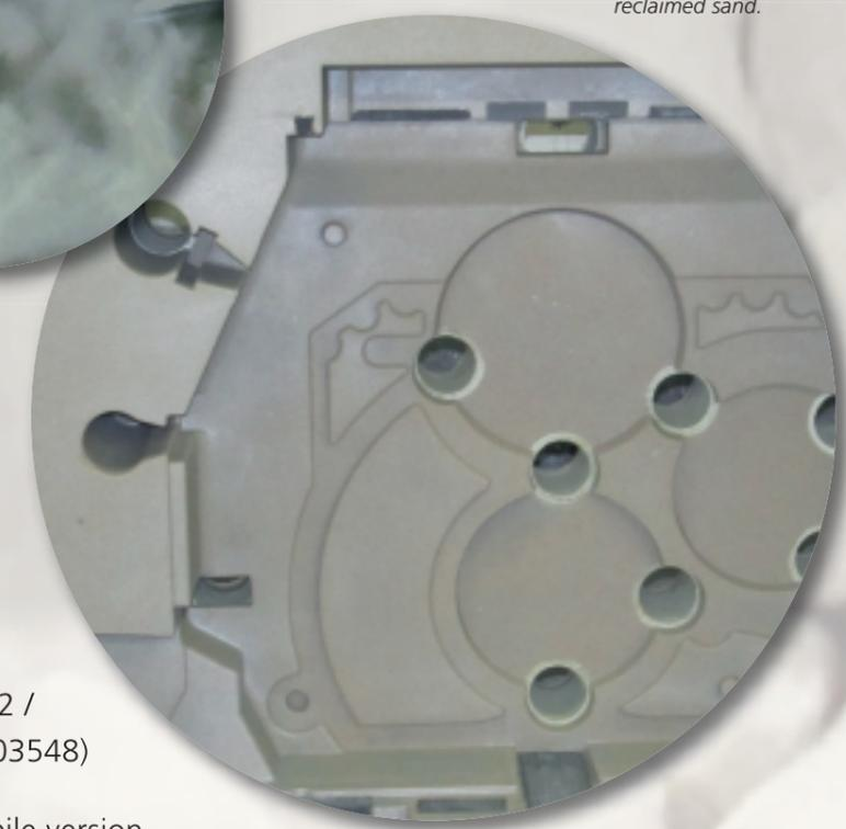
Mould manufactured with 80% reclaimed sand.
